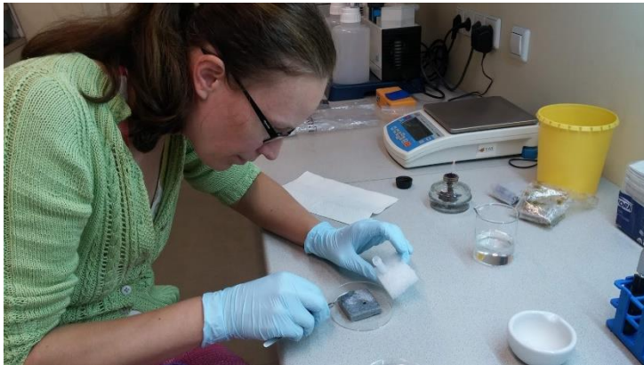
Removal of biofilm from tiles
