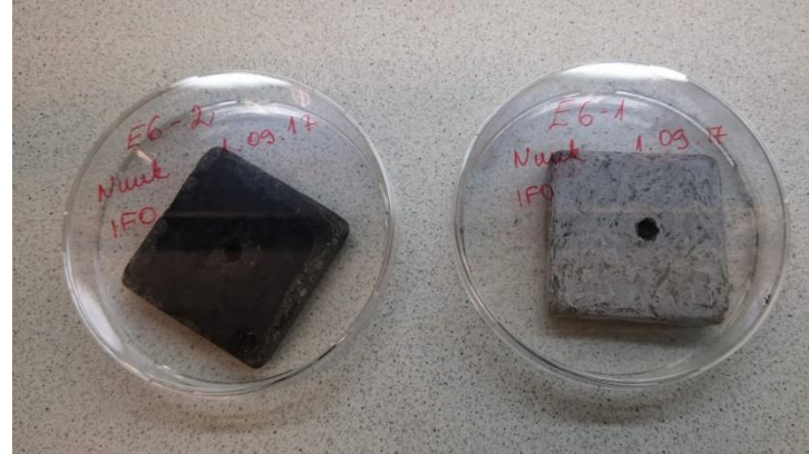
Removal of biofilm from tiles
